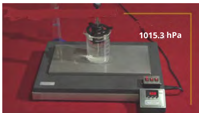
Figure 2: Digital hot plate with precision immersion thermometer for boiling point determination
