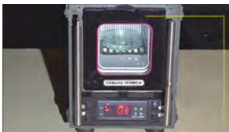
Figure 3: Programmable cold chamber for freezing point determination.
